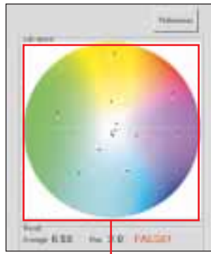
The values measured at the receiver's location are compared with those measured at the sender's location (contained in the JDF) and displayed.
