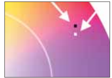
If a certain tolerance level is exceeded, the receiver's printout is evaluated as incorrect. If the customer's printout remains within the range of tolerance, the printout is evaluated as correct. The acceptable tolerance level is determined by the sender.
