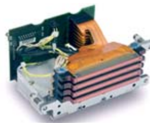
Competitive printhead array with 4 x 128 nozzles
