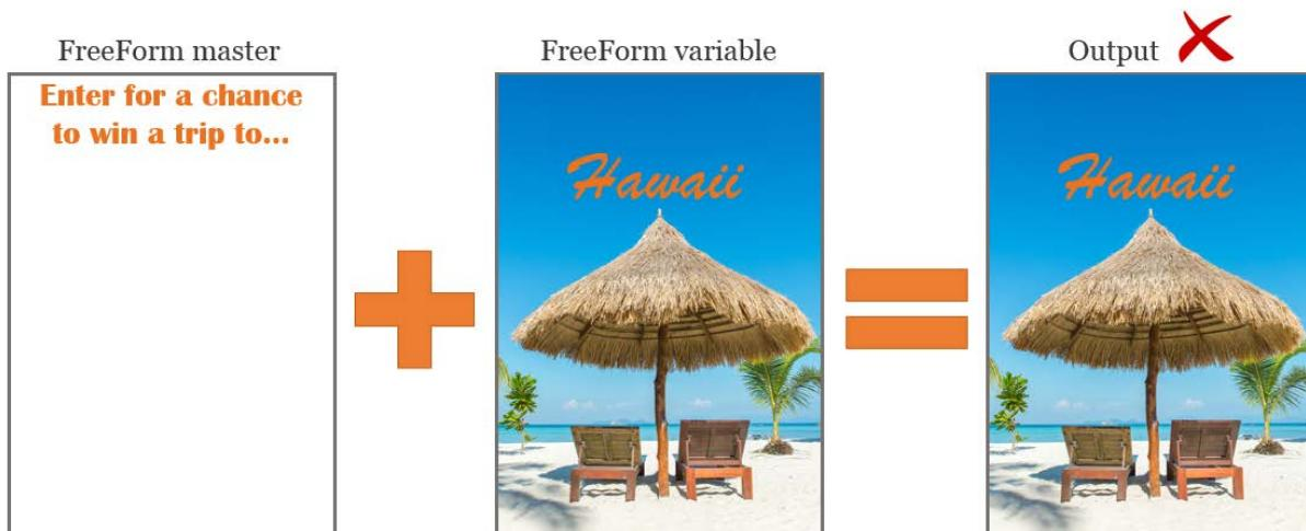
Variable content obscures the master content due to processing the master as a background layer
