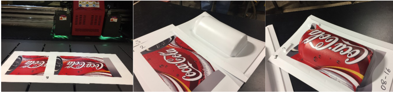
Thermoformed inkjet graphics produced at Joliet Pattern
