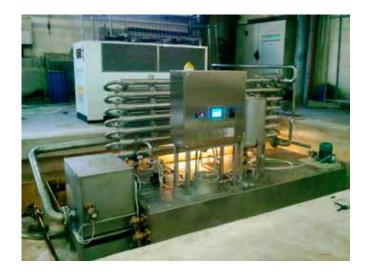
The Eco-Block is a compact device for preparation and recycling of the caustic soda lye for mercerizing machines. The Eco-Block is completely assembled as compact unit, tested and ready made for connection to all utilities. The standard Eco-Block can supply caustic soda lye for two mercerizing machines type Extensa. For more machines it requires increased cooling capacity.
