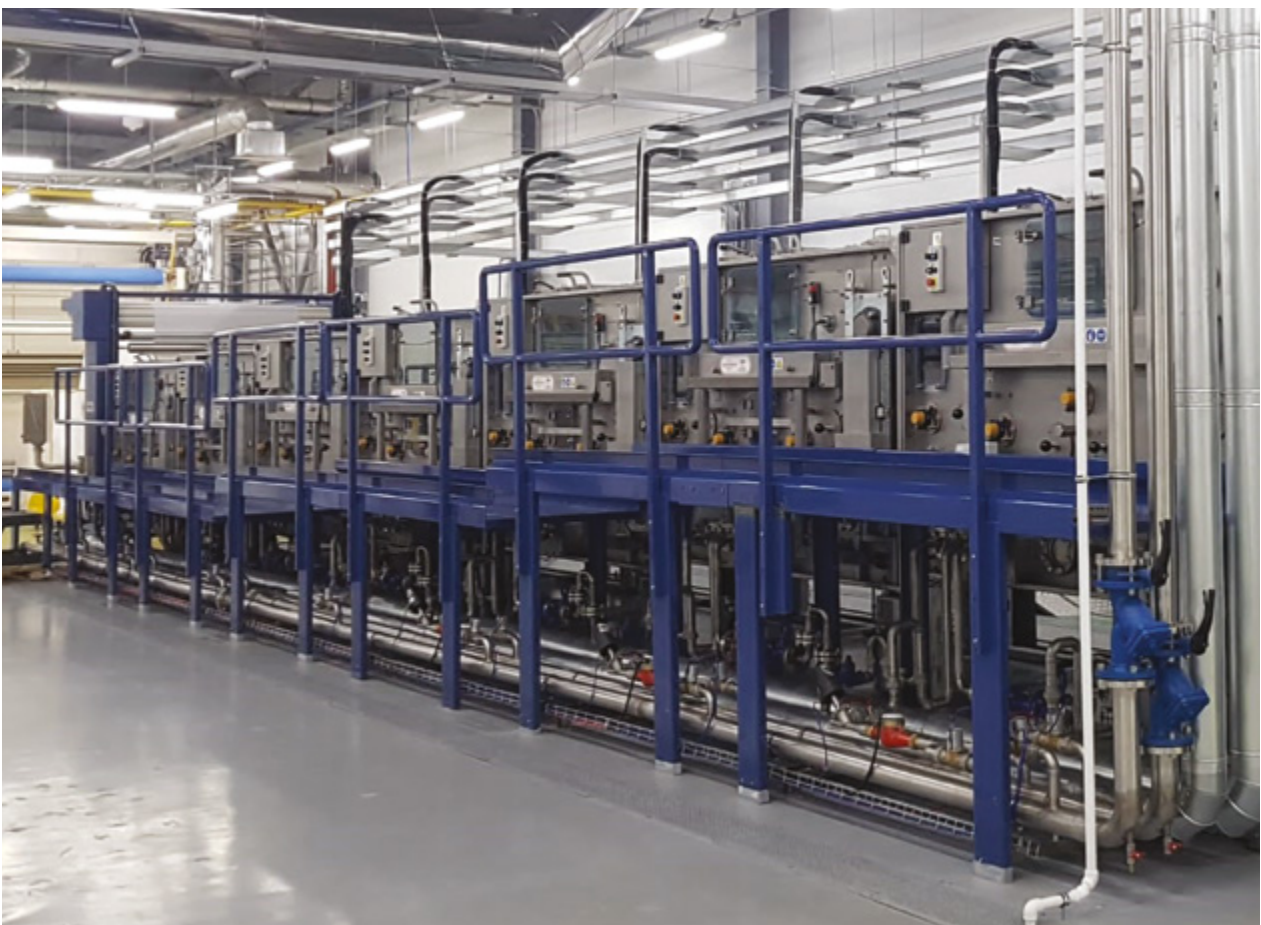
This solution increases the washing effect dramatically, facilitating the removal of glues like PVA, ACRYLIC, CMC, and, when performed in combination with enzyme HT amino-acid glues as well.
