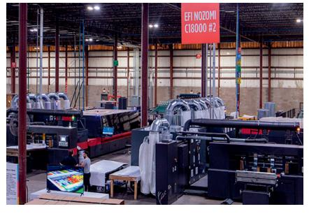
C18000 prints high-end, direct-to-board production at speeds up to 246 linear feet per minute, or approximately 10,000 35x35-inch boxes per hour two up. It is a groundbreaking production device that has earned multiple industry awards for its high quality, efficiency and productivity.
