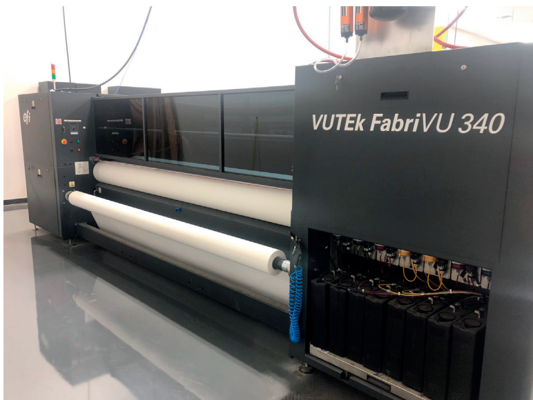
The EFI VUTEk FabriVU 340 allows George P. Johnson to quickly switch between printing direct-to-fabric or on transfer paper using the same inkset, giving operators more flexibility in their output.
