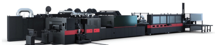
The EFI Nozomi 14000 LED offers high-speed single-pass corrugated production with print speeds up to 328 linear fpm.
